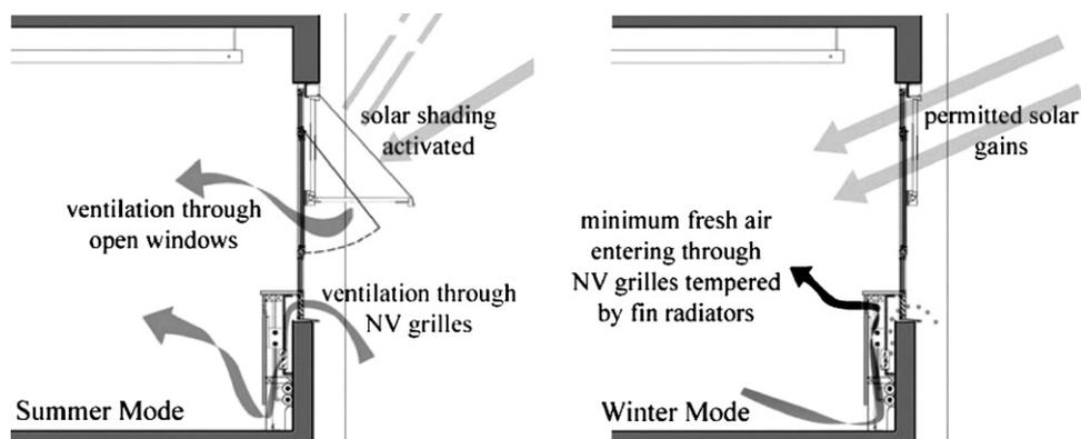
Fig. 2. Typical window section in the surveyed building showing ventilation strategy.
