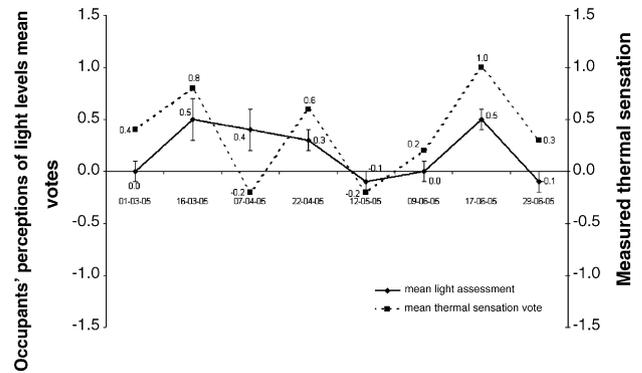
Fig. 7. Occupants’ perceptions of lighting levels mean votes and measured thermal sensation.
