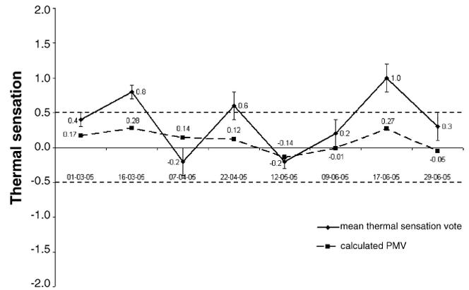
Fig. 4. Occupants' mean thermal sensation vote and calculated PMV values.
