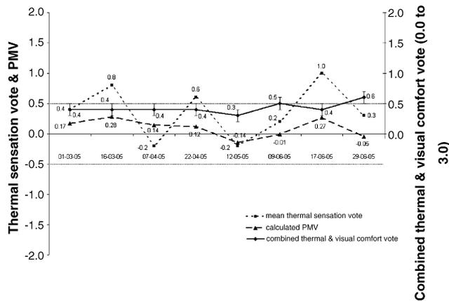
Fig. 8. Combined mean thermal and visual comfort vote, mean thermal sensation vote and calculated PMV.
